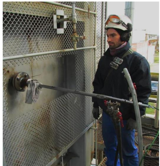
*Temperature measurement inside a heater using a suction pyrometer*
